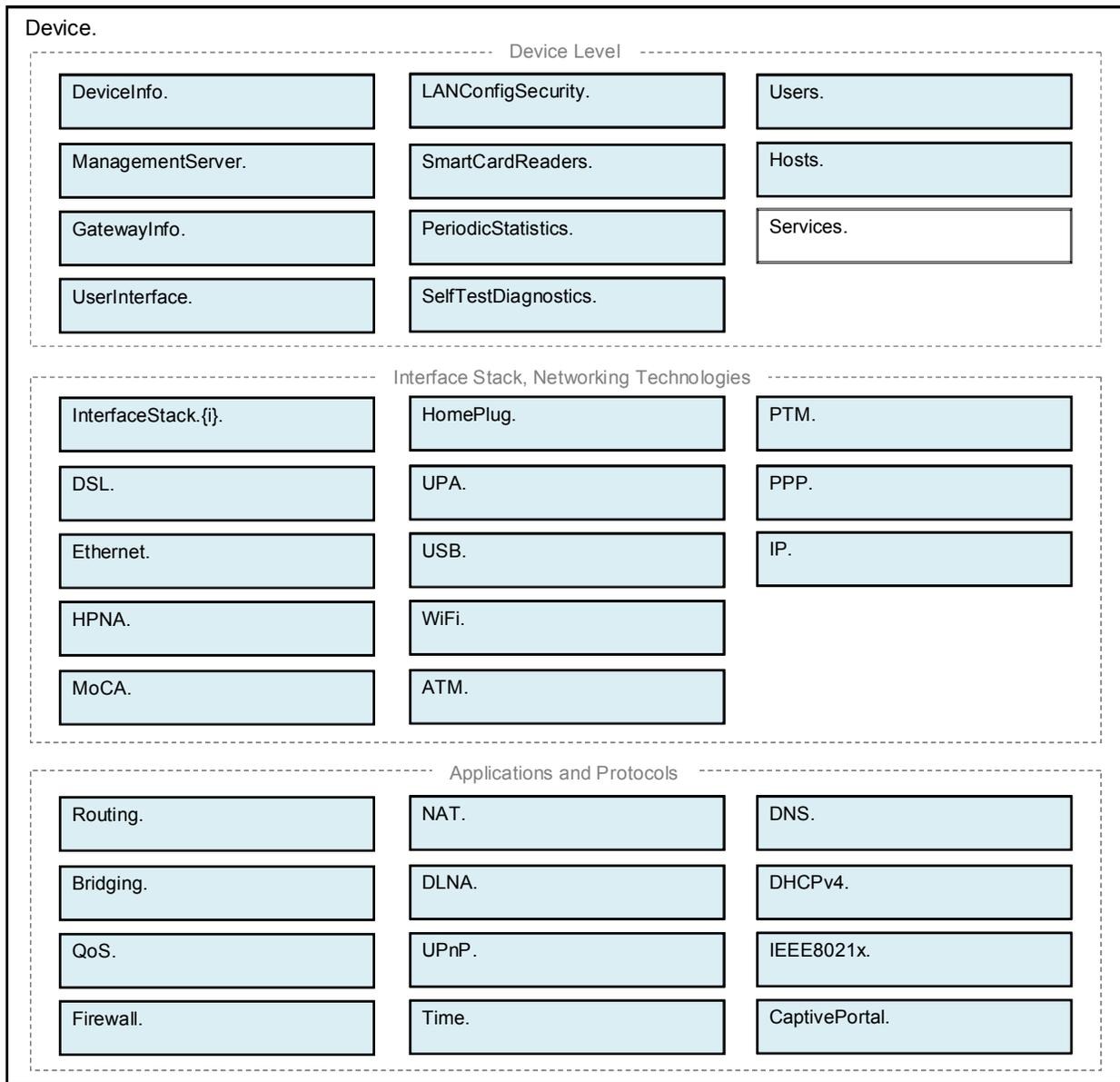
**Figure 1 – Device:2 Data Model Structure – Overview**
