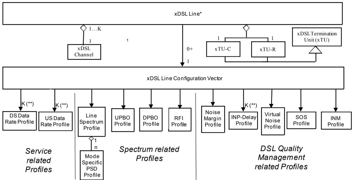
\* Note: in direct attachment method mode, the xDSL Line is equal to the xDSL Line Configuration Vector.
