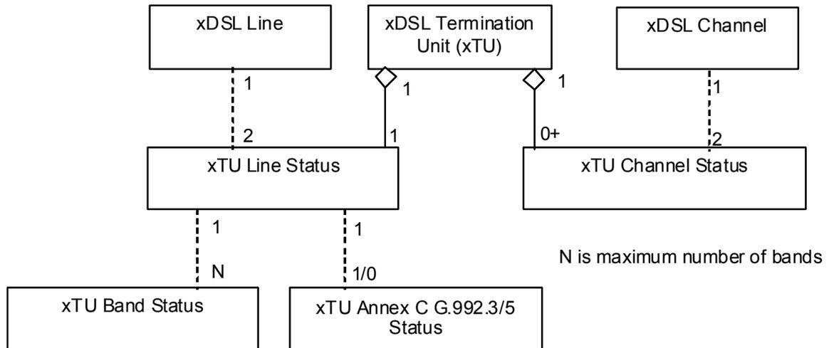
**Figure 3/TR-252 - Managed object model: xDSL status monitoring**
